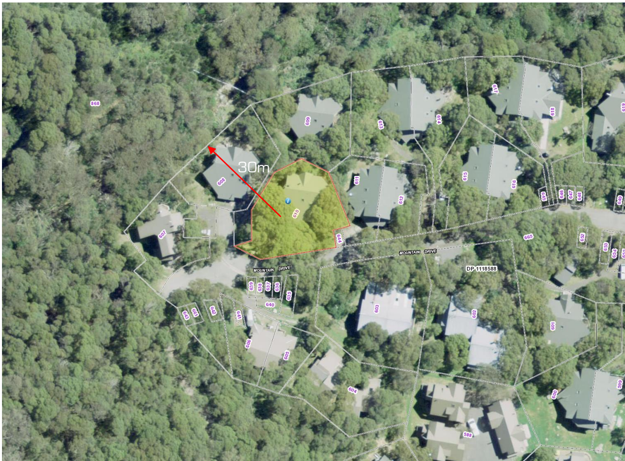
Figure 10: Aerial view demonstrating the distance between the closest unmanged vegetation with a continuous canopy to the proposed additions and external alterations
